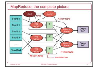
Step 1: Split input files into chunks (shards) • Break up the input data into M pieces (typically 64 MB) Shard 0 Shard 1 Shard 2 Shard 3 Shard M-1 Input files Divided into M shards
