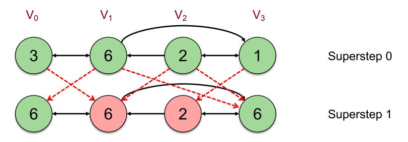
Superstep 0: Each vertex propagates its own value to connected vertices
