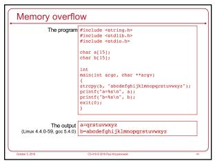
Memory overflow · We may be able to overflow a buffer and overwrite other variables in higher memory For example - Overwrite a file name
