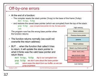
Off-by-one errors · Stuff the buffer with · Local variables • "saved" %rbp (can be garbage) • "saved" %rip (return address) High memory · Malicious code, pointed to by "saved" %rip - When the function's calling function returns It will return to the "saved" %rip, which points to malicious code in the buffer ed rbp (frame pointer char buf[128] MALICIOUS CODE
