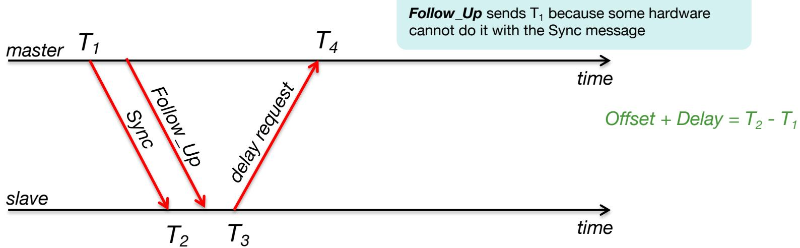
Slave needs to figure out the network delay. Send a *delay request*
