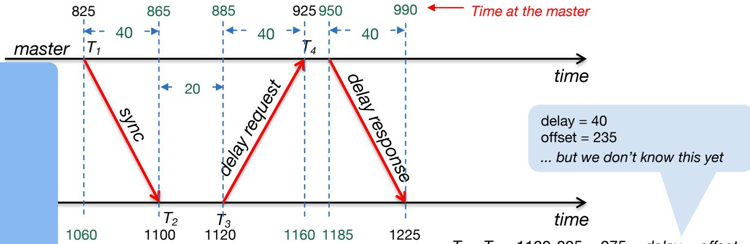
$$T_2 - T_1 = 1100 - 825 = 275 = \text{delay} + \text{offset}$$
