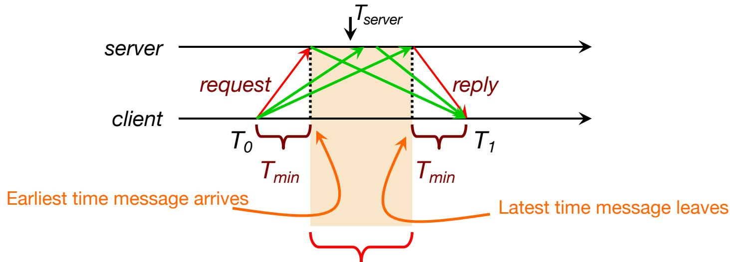
$$\text{accuracy of result} = \pm \frac{T_1 - T_0}{2} - T_{min}$$
